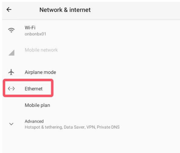
In the "Ethernet" interface, "dhcp" is displayed by default, and IP addresses are automatically assigned. If you need to change the IP address, you can click "Ethernet IP mode" to change the IP acquisition method. Change "Ethernet IP mode" to "static," then click "IP address" in the pop-up window to make the changes. After making the changes, click "OK" to complete the IP address modification.
