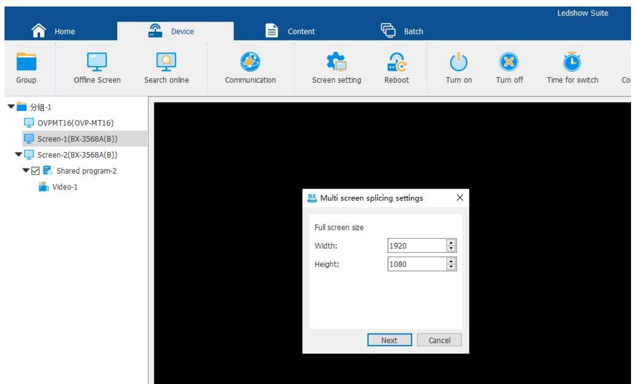
If the two screens to be tiled have a width of 1920 and a height of 1080, and they need to be tiled horizontally, add the width values together to get 3840, leaving the height unchanged. In the multi-screen tiled interface, enter 3840 after the width and 1080 after the height. Click "Next".
