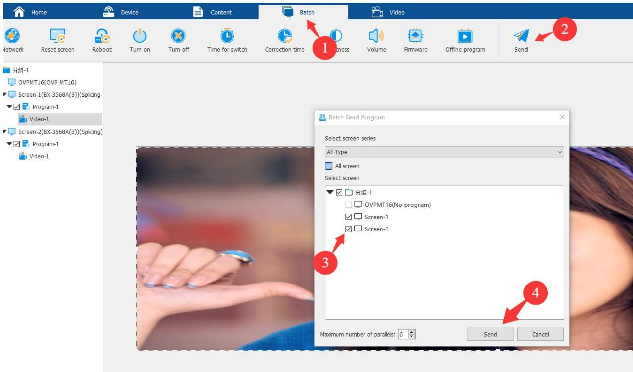
On the main interface, select the program under the screen that is the main screen, click "Batch" and then click "Send", check the two cards to be spliced, and finally click "Send". Group sending is required .
