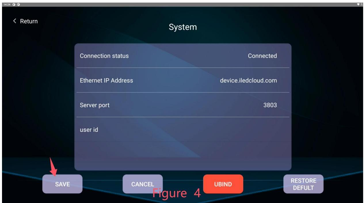
After clicking "Save" in Figure 4, the binding is successful. Exit to "Figure 1" and log in to the cloud platform to find this device.
