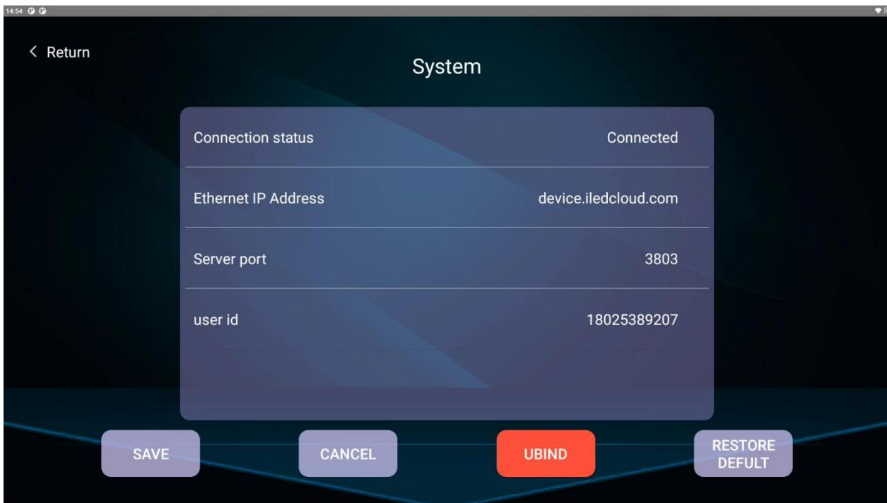
Add the mobile phone number or email address used when registering with the cloud platform to the "user id" field, then click "OK", and then click "SAVE" to successfully bind the account .
