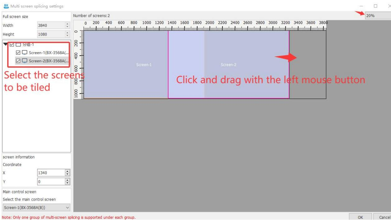
Once all the screens that need to be spliced have been dragged to the appropriate positions, click "OK" in the lower right corner to complete the splicing settings.
