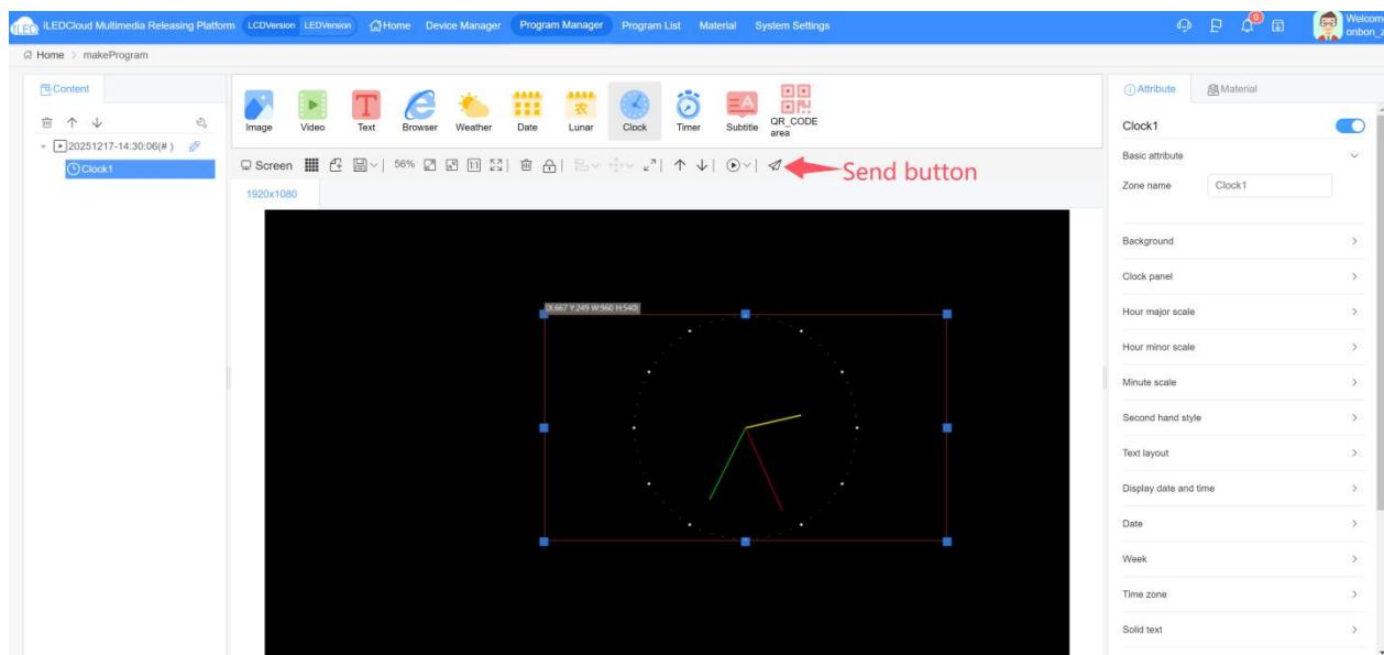
In the pop-up dialog box, click "OK" and enter a name in "Name". A selection interface will appear to choose the controller to send to. Select the controller and click "Release" to send successfully.
