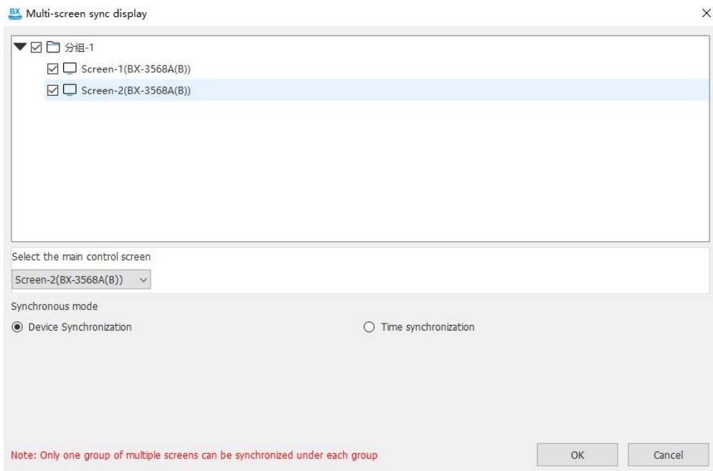
On the main interface, select the program on the screen that is the main screen, click "Batch" and then click "Send". Select the two cards to synchronize, and finally click "Send". Group sending is required .
