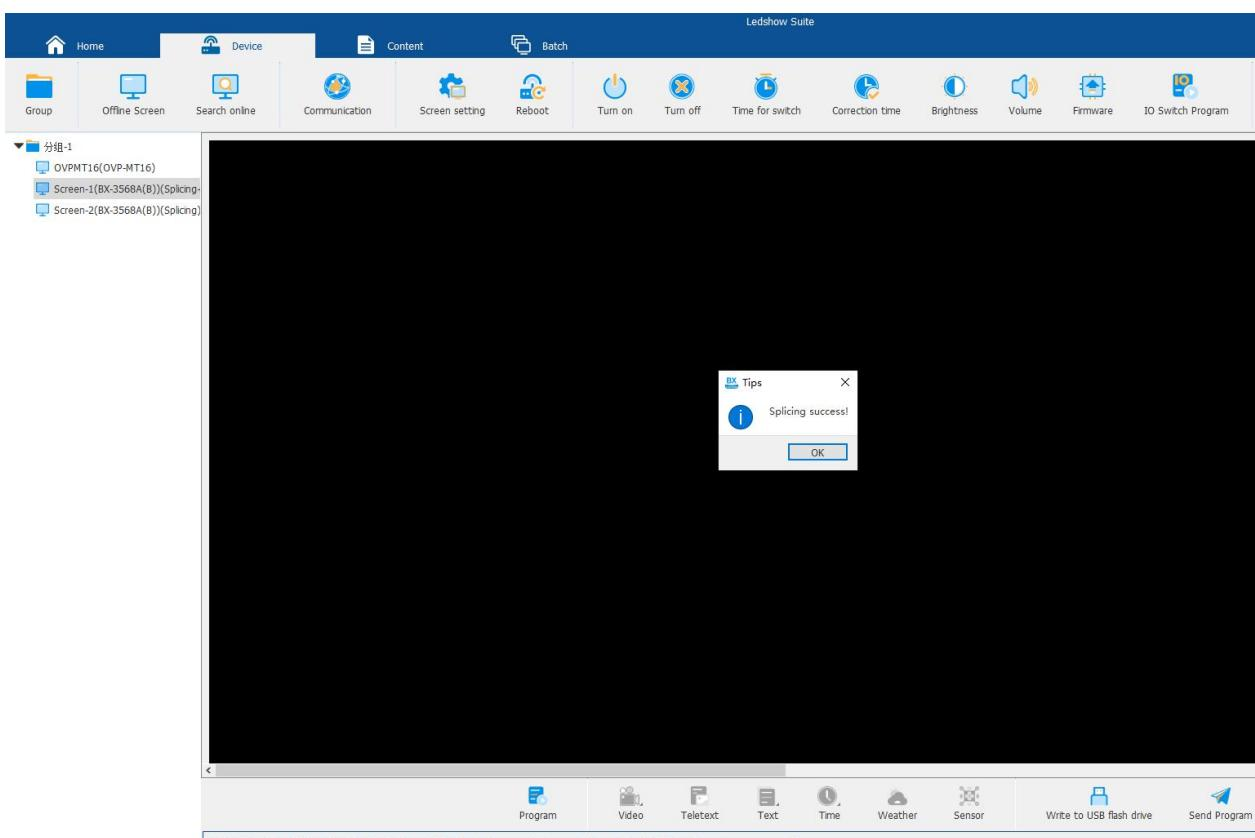
On the main interface, first select the main screen that needs to be spliced, add a program, such as adding a text and image area, and then right-click on the program preview interface and select " Enlarge ".
