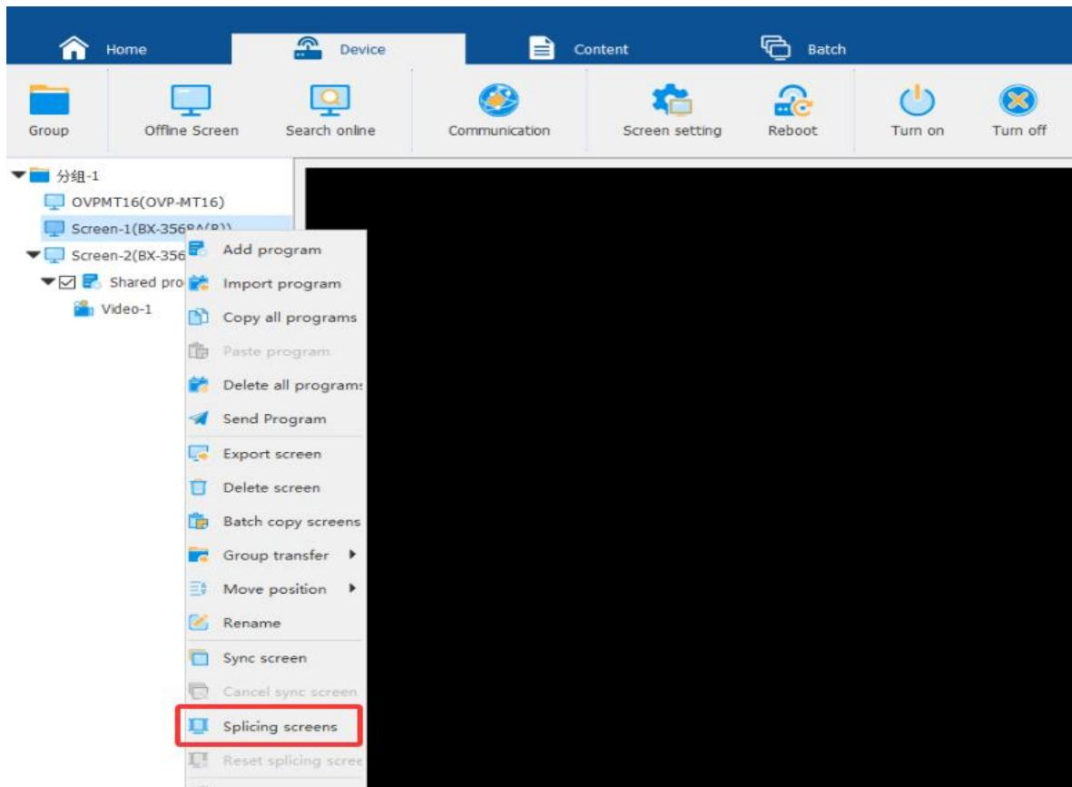
In the pop-up multi-screen splicing interface, you can enter the total width and total height of the two screens that need to be spliced.
